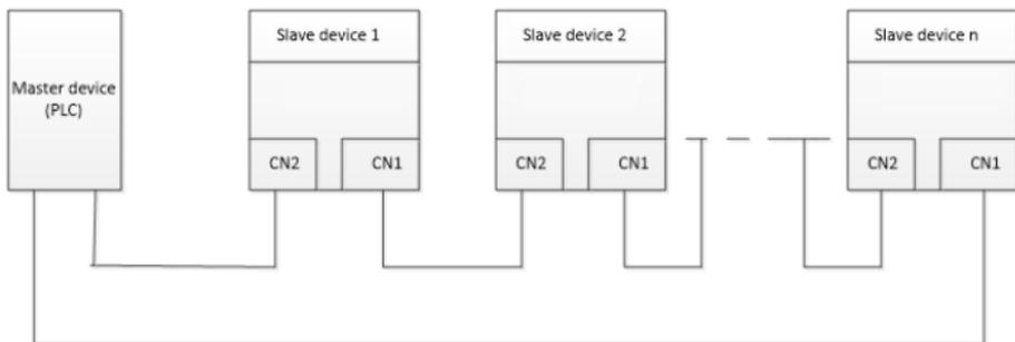
Figure 0-2 Electrical wiring diagram for a linear topology
