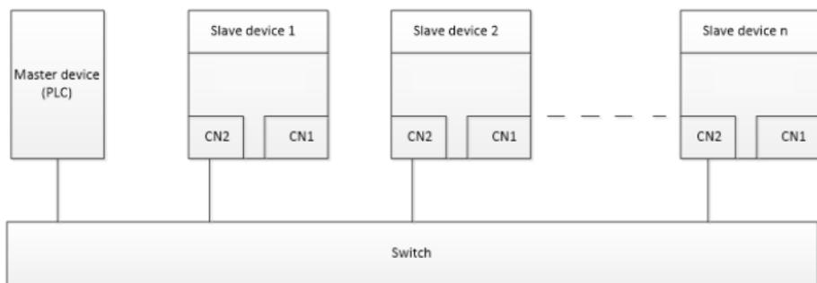
Figure 0-3 Electrical wiring diagram for a star topology
