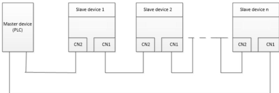
Figure 0-4 Electrical wiring diagram for a ring network
