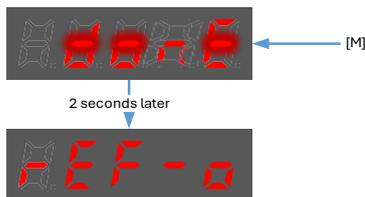
Step 7 Press the **[◀]** key to return to the utility function mode display Fn003.
