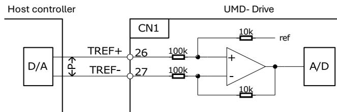
**NOTE** P represents a twisted-pair cable. To suppress noise, be sure to use twisted-pair cables.
