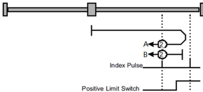
**Methods 3 and 4: Using C pulse and positive reference switch**
