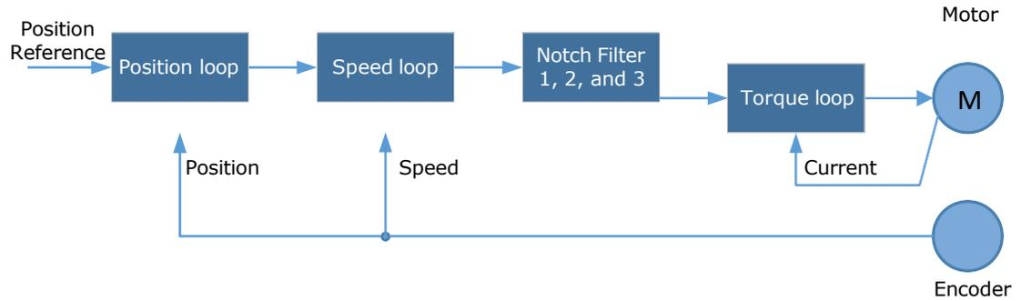
Figure 8-19 shows the relevant parameters for the notch filter. Since the notch filter can attenuate the signal at the notch frequency, if you set a proper frequency (Pn181, Pn184 or Pn187), depth (Pn182, Pn185 or Pn188) and width (Pn183, Pn186 or Pn189), the vibration signal in the torque reference can be filtered.
