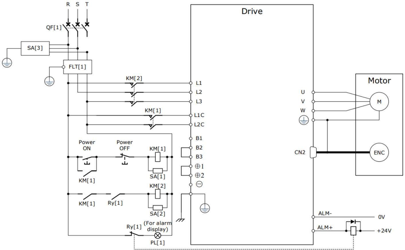
The following figure shows the wiring example for using the single-phase AC input power.
