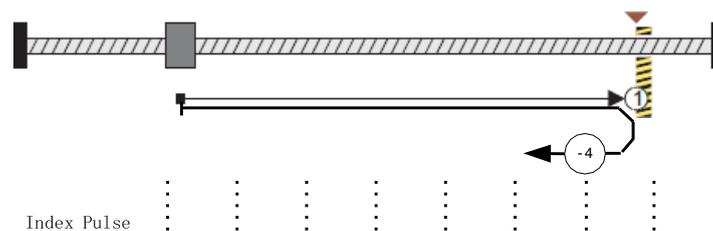
**Movement in negative direction, hitting an end and reversing to travel, the target homing position is the C pulse**
