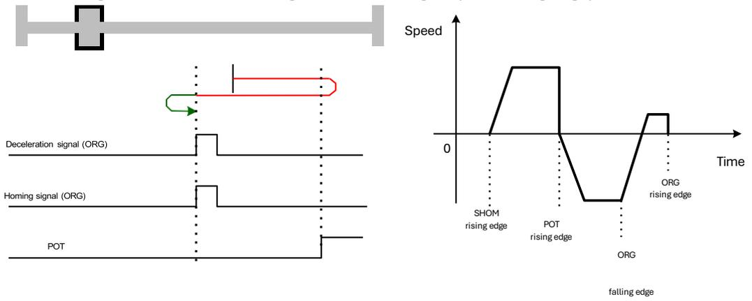
Homing modes 3 and 4, using deceleration point as ORG switch, and origin as Motor's Z signal
