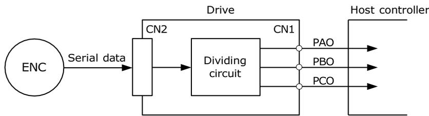
**Note:** Even in the reverse mode (Pn001.0=1), the pulse dividing output phase form is the same as the standard setting (Pn001.0=0).
