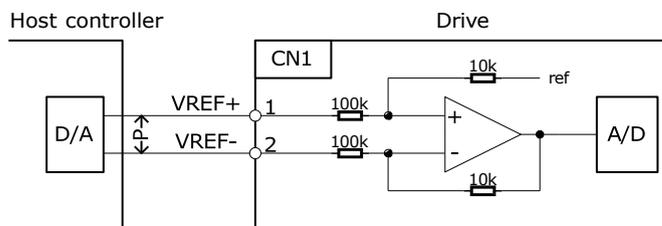
**NOTE** “ P ” represents a twisted-pair cable. To suppress noise, be sure to use twisted-pair cables.
