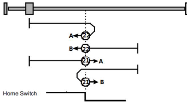
Methods 33 and 34: Homing by using C pulse
