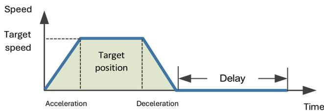
The position planning during Interrupt is to plan the position reference on the basis of the original reference speed.
