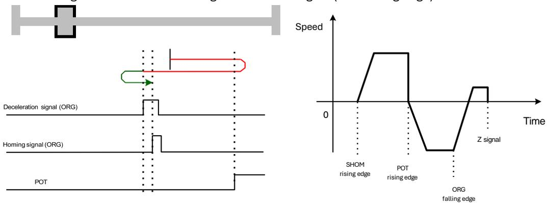
**Homing modes 5 and 6, using origin as motor's Z signal**
