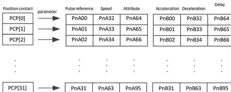
The pulse reference defines the number of pulses of the contact, the speed defines the running speed of the contact, the attributes defines the motion attribute of contact, the acceleration and jerk define the acceleration/deceleration of the contact, and the delay defines the delay time after the contact reference is sent.
