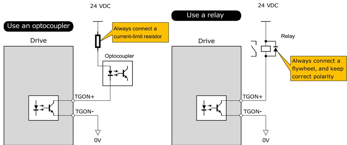
The maximum permissible voltage and current of the optocoupler output circuit inside the servo drive are as follows: Maximum voltage: 30 VDC
