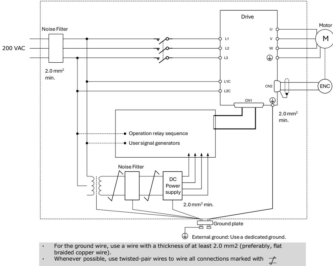
**Noise Filter Wiring and Connection Precautions**
