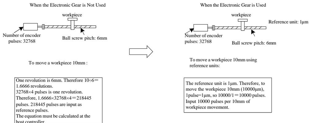
If the mechanical reduction ratio between the motor shaft and the load side is set to m/n, the setting value of the electronic gear ratio can be calculated according to following formula. (When the servomotor rotates m revolutions, the load shaft rotates n revolutions)
