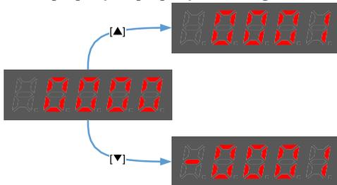
**NOTE:** the offset can be adjusted from -1024 to 1024.
