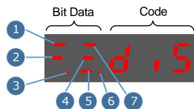
The display meaning of each segment on Bit Data are shown in Table 4-1 , and they have different meanings under Speed or Torque Control Mode and Position Control Mode
