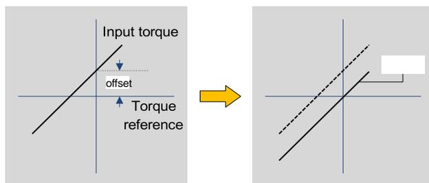
**Auto Adjustment of the Torque Reference Offset**
