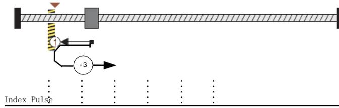
**Method -2: Movement in positive direction, hitting an end, makes the current position for the homing point**
