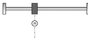
Method-4: Movement in positive direction, hitting an end and reversing to travel, the target homing position is the C pulse
