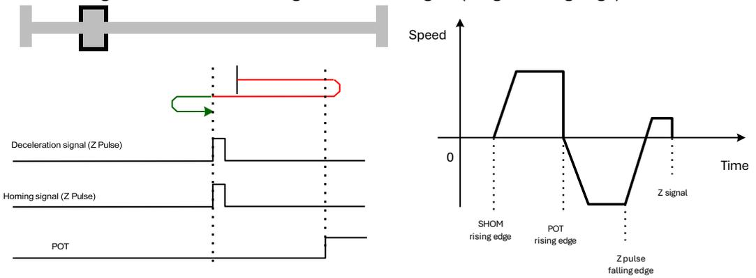
**Homing modes 7 and 8, using deceleration point and origin as overtravel switch**
