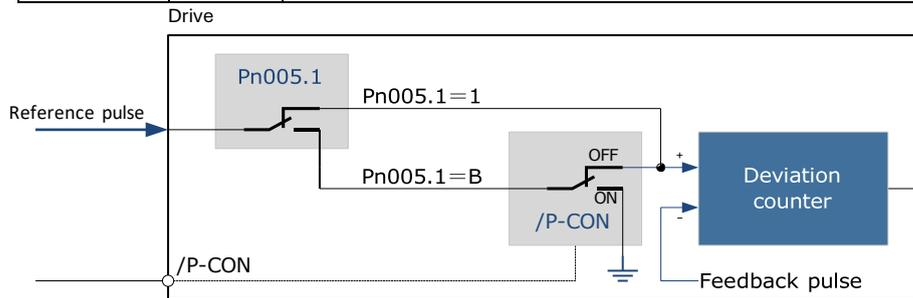
Inhibit (INHIBIT) is switched via /P-CON signal:
