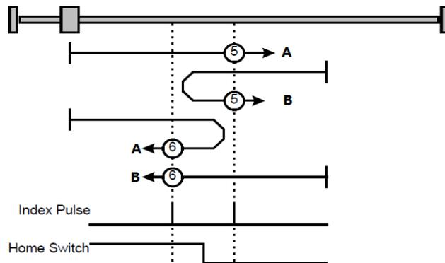
**Methods 7~14: Using reference switch , limit switch and C pulse**
