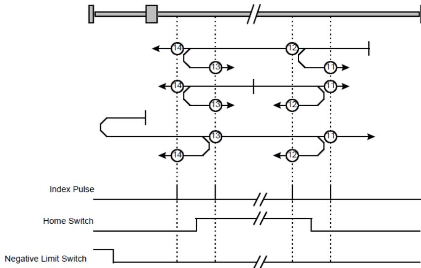
**Methods 17~20, 23~30: Not using C pulse**
