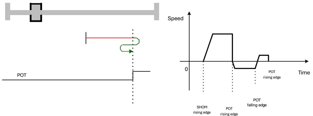
Homing modes 9 and 0, using deceleration point as overtravel switch, and origin as motor's Z signal
