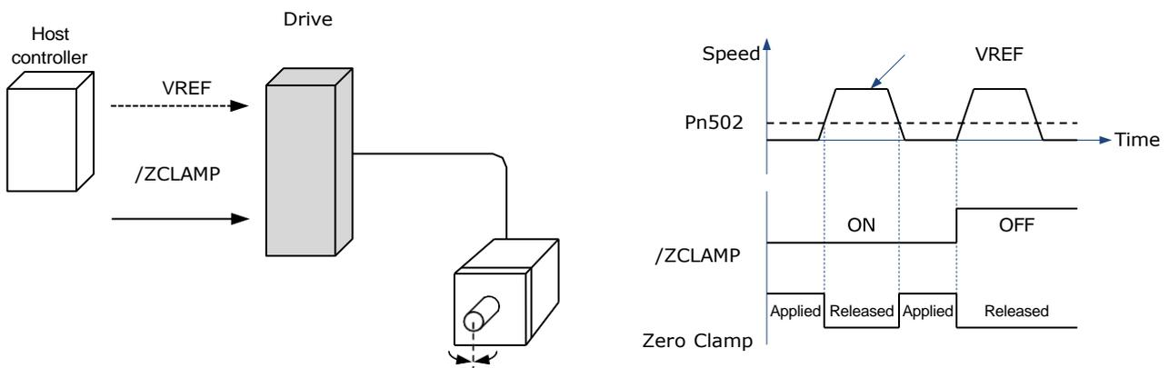
Adjust the position loop gain in Pn104 (position loop gain) if the servomotor oscillates in the zero clamp state. If the gain switching function is used, adjusting Pn109 (2nd position loop gain) is also required.
