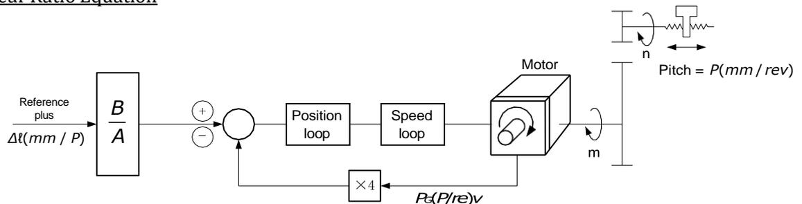
Where: Δl is the reference unit; P\_G is the encoder pulse; P is the pitch of the ball screw; m/n is the reduction ratio.
