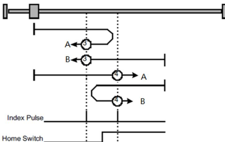
**Methods 5 and 6: Using C pulse and negative reference switch**
