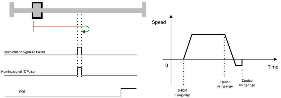
Hit the limit signal before encountering deceleration signal (Z signal rising edge).
