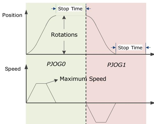
The Drive will operate the Motor repeatedly according to the parameter settings of the two operation patterns until you stop the program jogging operation manually.
