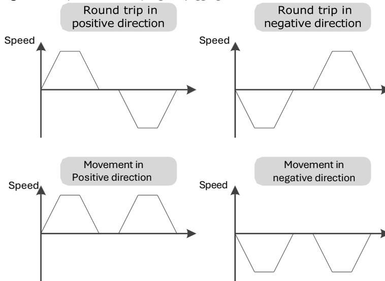
You should set the Rotations (Pn164 and Pn168) and Max Speed (Pn165 and Pn169) to a proper value. If the Rotations is set too small or the Max Speed is set too large, it is possible that the maximum speed set cannot be reached. In this case, it is necessary to increase the Rotations or decrease the Max Speed.
