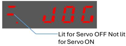
Step 4 Press [M] key to Servo ON (supply power to Motor).
