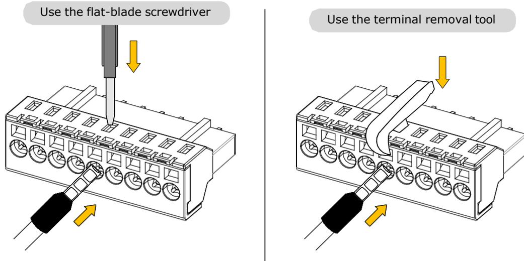
Step 6 Insert the crimped cable into the connection terminals, and then pull out the tool.
