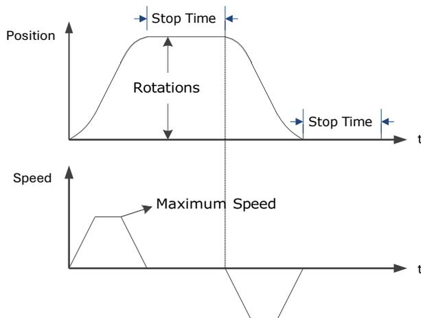
The Drive will operate the Motor repeatedly according to the parameter settings of the two operation patterns until the tuning is completed. You can set the parameters Pn164 and Pn168 to a negative value for reversing the Motor, so that there are four ways of the operation in the program jogging, as is shown in Figure 8-9.
