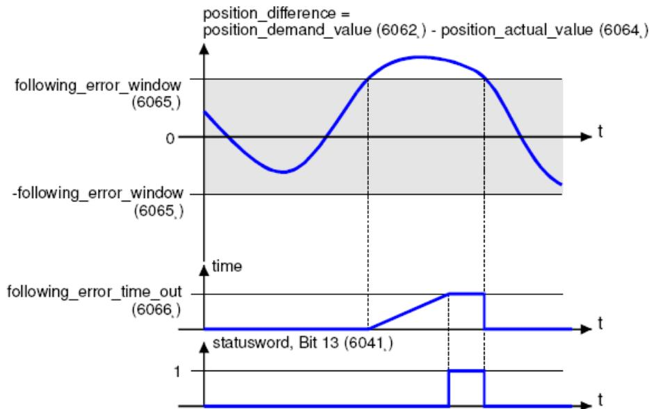
The deviation of the actual position value (position\_actual\_value) from the desired position value (position\_demand\_value) is named the following error. As shown in figure above, if for a certain period of time this following error is bigger than specified in the following error window (following\_error\_window) bit 13 (following\_error) of the object status word will be set to 1.
