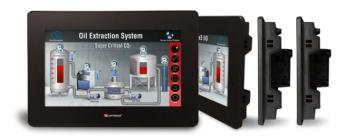
in Standard (B5) and Pro (B10) models. Both models support advanced communications, including MQTT, VNC, FTP, SNMP, email and SMS messaging. The Pro version also offers built-in Webserver, video support and SQL.
