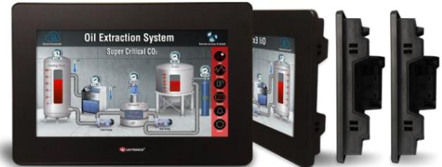
UniStream Built-in benefits include auto-tuned PID, data logging, data tables and recipes, data sampling displayed via built-in Trends and Gauges, Alarms, multi-level passwords, portrait mode, and plug & play communications for CANopen, CAN Layer2, MODBUS, EtherNet/IP, Servo made Simple, and more.
